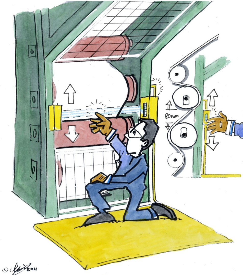
Fig. 2: The rollers are moved apart when the light beam is interrupted
