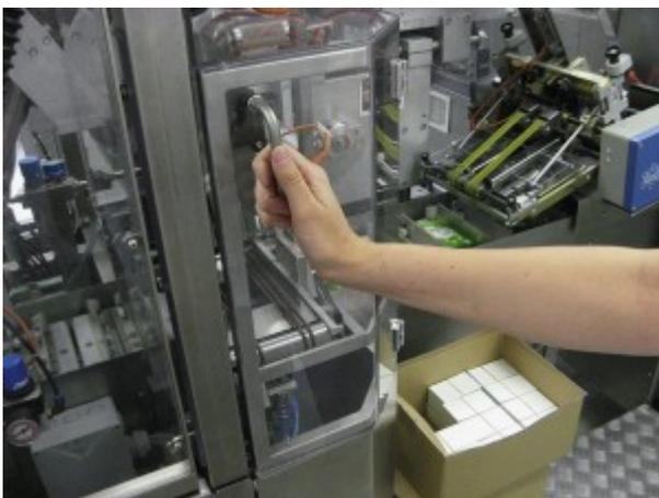
If you have found out that protective equipment in your company has been defeated, it is time to take action. After having taken immediate measures to restore the safe (original) condition of the machine, it is necessary to systematically analyse the situation that was the cause for defeating the protective equipment.
